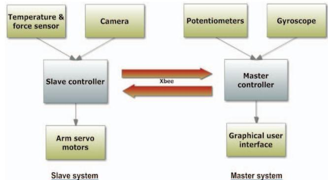
Fig. 1: Block diagram of the Master-slave system
