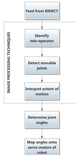
Fig. 9 Block Diagram of Arm Control using Kinect
