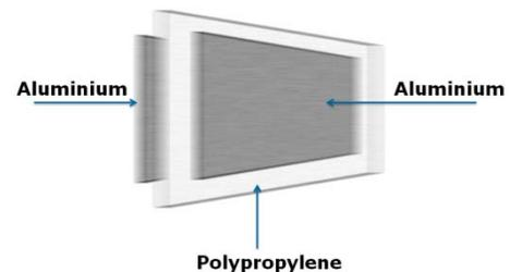
Fig. 4 Chassis of the robot
