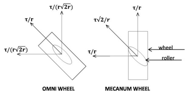
Fig. 5 Vectors representation of force acting on mecanum wheel
