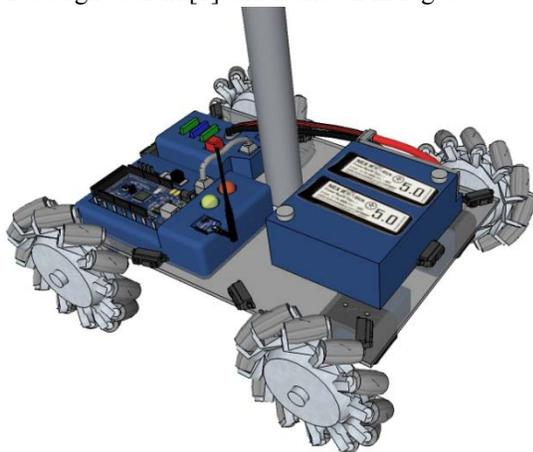
Fig. 3 3D model of Chassis and Mecanum wheel drive
