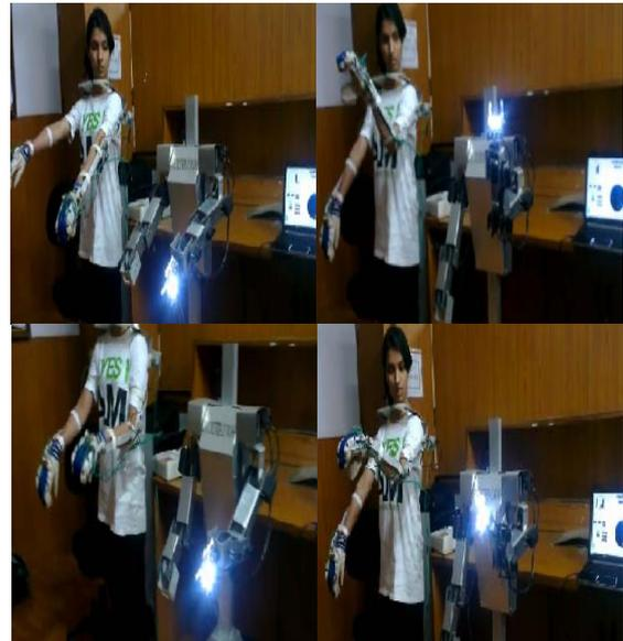
Fig.14. Mimic operation of robotic arm
